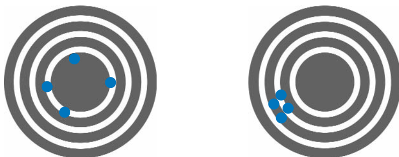
Figure 1 Accuracy and precision. left: High accuracy but low precision; right: High precision but low accuracy.
