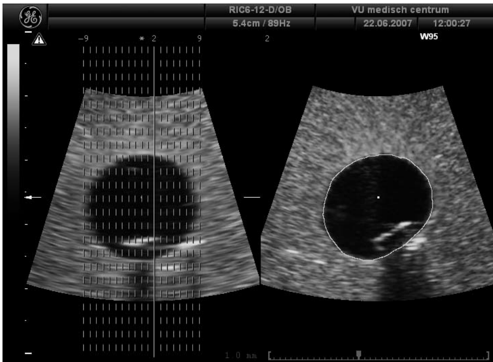
Figure 2 The three-dimensional slice method applied to a static volume of a miniature balloon model, showing the manual trace used to outline the contour of the balloon.
